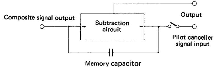
In order to simplify the operation theory, the composite signal component is given only as a low frequency signal and a pilot cancel signal has the same phase, same amplitude as the pilot signal in the composite signal.
