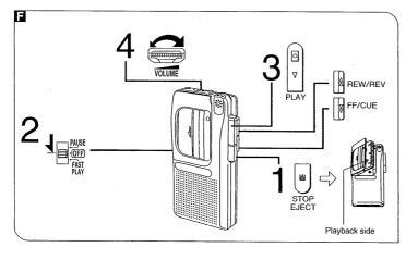
To stop recording Press STOP/EJECT.
